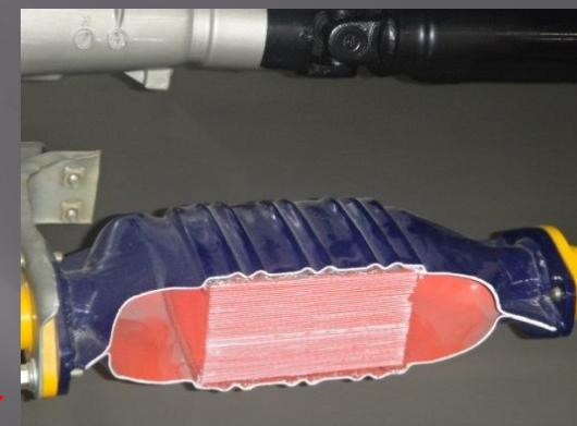
Electro-Catalytic Honeycomb (ECH)
